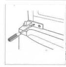
11. Place the upper door back on. Ensure the door is aligned horizontally and vertically so that the seals are closed on all sides before finally tightening the top hinge. Then insert the hinge and screw it to the top of the unit.
